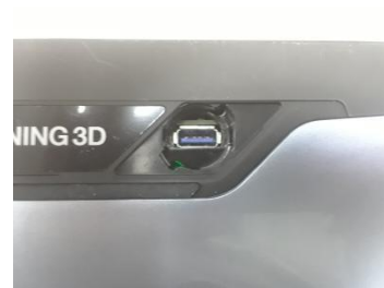
USB port for add-ons (Output voltage and current:12V/500mA)
