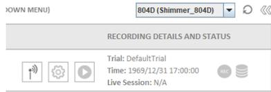
Step 3: Once you select your Shimmer Device from the top right drop down menu, click the button on the bottom left to initialize a connection and the play button to visualizing readings
